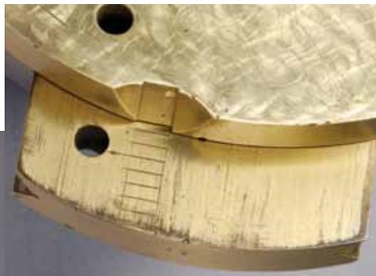
(Detail above) The eccentricity scale is engraved on the back at the bottom of the chuck. Two holes allow a tapered pin to be inserted, locking the eccentric chuck in its centered position.
