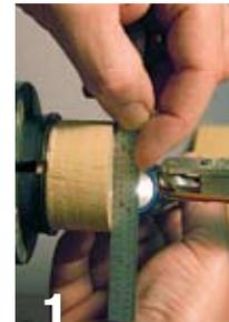
**1** Check flatness with a light source from behind (a flashlight is used here) and a straightedge to help identify any high or low spots.
