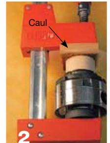
**2** While the workpiece is still in the chuck, use a caul (MDF in the photo *above*) to clamp the assembly. A layer of heavy plastic keeps glue off the caul and clamp.
