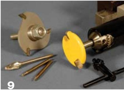
**9** Using materials available today, a flex-shaft handpiece can be adapted to be held in the sliderest, thereby allowing use of various router bits and slotting cutters. From experience, burrs, like those pictured *lower left*, do not produce desirable patterns and should be avoided.
