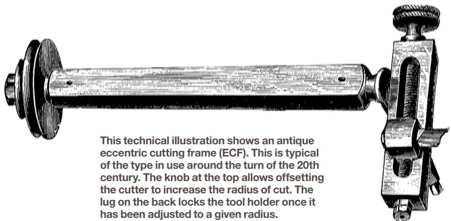
This technical illustration shows an antique eccentric cutting frame (ECF). This is typical of the type in use around the turn of the 20th century. The knob at the top allows offsetting the cutter to increase the radius of cut. The lug on the back locks the tool holder once it has been adjusted to a given radius.
