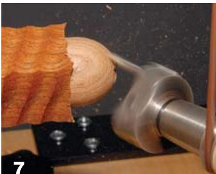
**7** With chips flying, a modern eccentric cutting frame (ECF) uses an  $\frac{1}{8}$ " round carbide cutter. An example of the ECF's versatility is that it can cut a variety of hemispherical shapes merely by introducing it to the work at an angle, shown here at about 45 degrees.
