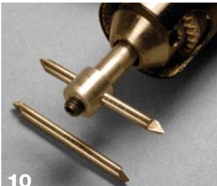
**10** This is a simple design for a cutter to hold round carbide split-end blanks, reshaped and sharpened as desired. This one is a 1/8"-diameter cutter with a 60-degree point. From readily available blanks, cutters can be made in a variety of sizes.
