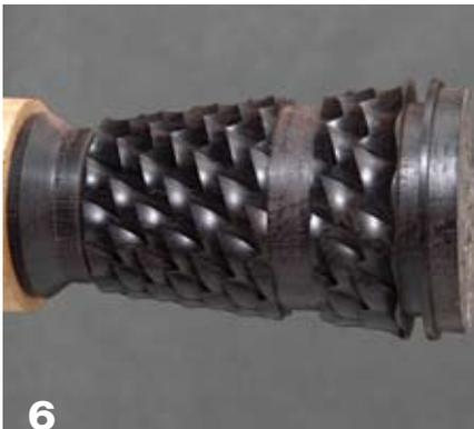
**6** A surprising range of patterns can be created with the UCF simply by tipping it at angles. This pattern was produced using a rose-engine lathe and the UCF tilted to about 30 degrees.
