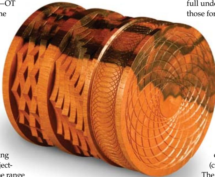
This ornamental turning sample shows just two variations of the thousands possible on the basket-weave pattern. The left is a simple alternating pattern; the right a pseudo-spiral effect. The face and the right end show two types of circular cuts possible with the eccentric cutting frame (ECF). The cut on the side of the cylinder has been "beaded" first with the ECF, then decorated on the resulting curved surface with additional circular patterns.
