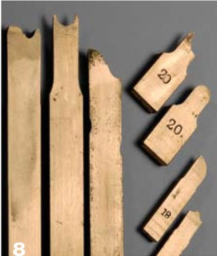
**8** Period cutters from the heyday of OT include large-size cutting frame cutters, *top right*, stamped to indicate their 0.20" width. The small-size cutting frame cutters, *bottom right*, are often referred to as ECF cutters, as ECFs typically did not accommodate the larger sizes. The left three cutters are elaborately profiled examples of special cutters used as fixed tools in the sliderest.
