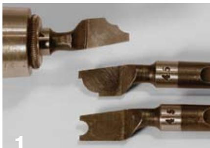
Examples of antique ornamental drills. Note the variety of profiles among these antique ornamental drills. These are all slightly offset, or cranked out, so that as they revolve, they only cut from the centerline out. The inside corner of each tip is exactly aligned with the centerline of the drilling spindle.
