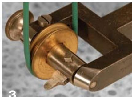
A roundnose cutter is installed in this antique vertical cutting frame (VCF).
