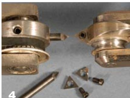
Two examples of horizontal cutting frame (HCF) cutter heads are shown above. Both have 60-degree tips appropriate for rose-engine work. The motorized version, left, uses 1/8" round carbide cutters. The belt-driven version, right, uses triangular carbide inserts borrowed from the metalworking industry.
