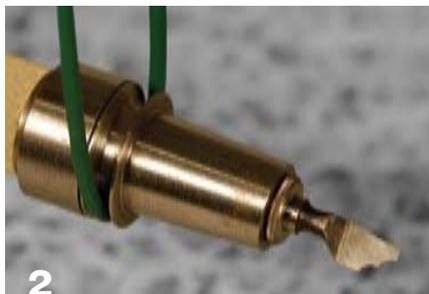
This is the typical nose of a drilling spindle with a drill in place. The belting connects to the overhead drive.
