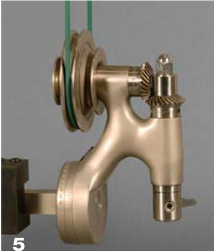
**5** This universal cutting frame (UCF) is styled after the original design by Birch. The bevel gears on this model allow the belt to remain directed upward to the overhead drive while the cutting head can be tipped through various angles between horizontal and vertical.
