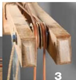
Two inexpensive sliding-glass-door wheels make perfect pulleys for the 1/8"-round belting. Crossing the belting provides a simple way to reverse the cutter direction.
