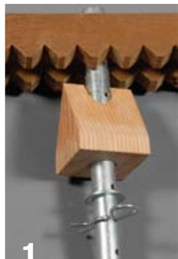
The notches on the underside of the arm allow adjustment on top of the pivot block, which is supported by a clevis pin. The washer between the two allows the arrangement to rotate freely.
