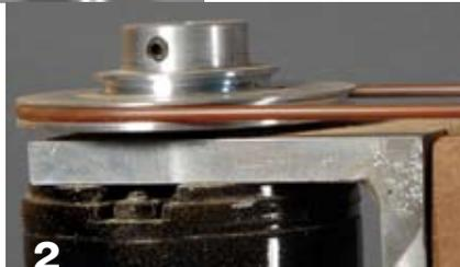
Even with a variable-speed motor, at least two steps in the pulley allow fine-tuning speeds. More steps would easily allow the use of a less expensive single-speed motor.
